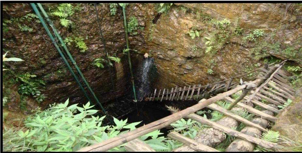
11: Precariously supported bamboo ladders going down to the rat holes. (Cement Factory: 31 May, 2010)
