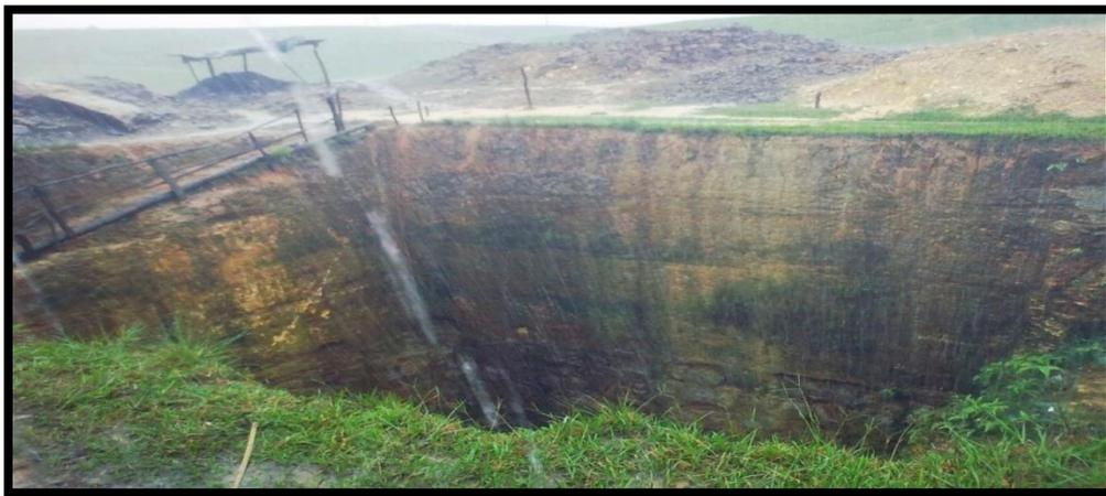
5: *Steep, sheer holes are punctured 100-180 ft. into the ground in the Myrsieng coal mine quarry. At the bottom of these pits, on each side of the walls, 'rat holes' are burrowed and laborers go digging inside these ratholes for coal. (7 December, 2009)*
